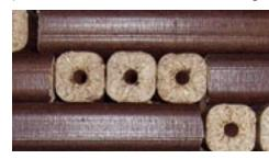
and the lignin contained in the wood can be softened, allowing it to act as a natural binder, producing a reformed log size product which should conform to European standard EN ISO 17225-3. Briquettes are dense which reduces the amount of storage space required and they're also clean to handle and easy to take home in 'ready to burn' retail packs.
