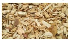
will help the appliance (especially domestic sized boilers) work at their optimum efficiency and reliability. Typical wood chip from a tree surgeon is too wet and variable in chip size for most appliances.
